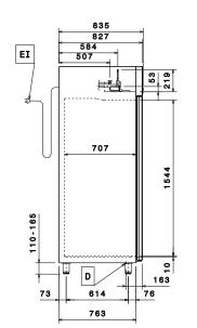
ED Remote electrical connection RO Refrigerant Outlet Electrical inlet (power) ΕI Refrigerant Inlet
